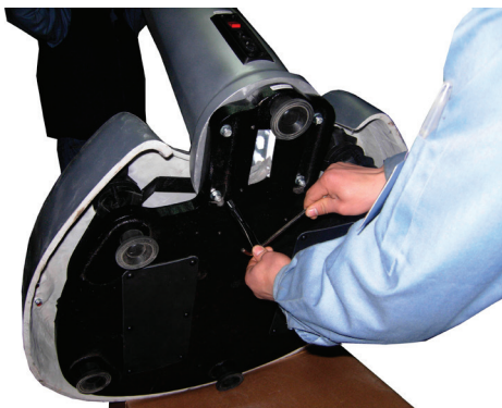
Pic #5 Tighten the column to the base
